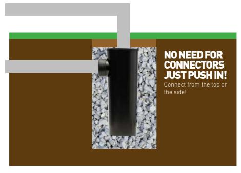
Can be installed into the top or through the side of the soakaway depending on where the pipework is situated.
