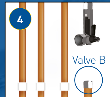
4 Slip on nut and olive to Valve (B).
