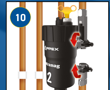
10 Tighten lid with the spanner provided and open the valves. Finally open the bleed valve to eliminate any air in the system.
