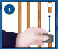
Cut 140mm of pipework.
