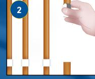
Slip on nut and olive on both sides.
