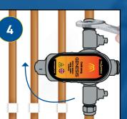
Once slid on, turn filter to right angle so you can tighten nuts.
